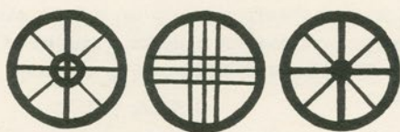
Three familiar patterns for the inner bracing of the smoke-hole frame.
